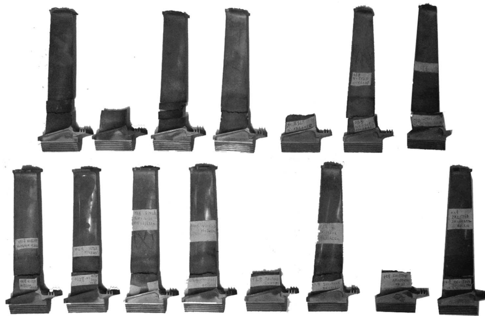
Fig. 7 Fracture blades of creep-fatigue tests
